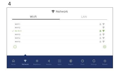
If an Internet connection is not found in Step 3, hold the power button for 3 seconds and release. This lets you enter the set-up page to find your Wi-Fi connection. Under the Network Tab, select the Wi-Fi network. Once connected, your device should start auto provisioning itself to your software provider. Once set up is complete, password **1elo** can be used to re-enter control panel if needed.
