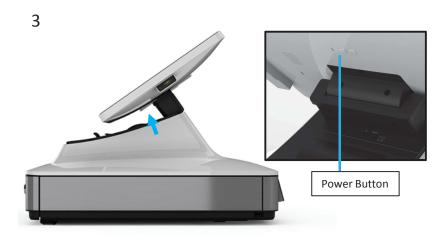
**Power on the register:** Press the power button (located on the back of the display head). If an Ethernet connection is available, registration will start automatically when the device powers on.
