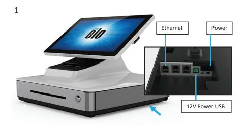
**Connect power and ethernet cable.** Connections are underneath the register near the back.
