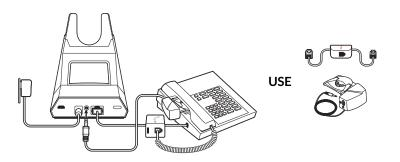
**IMPORTANT** *Cisco* phones use configuration **D** on the bottom of the base. Most other phones use default configuration **A**.
