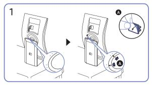
Attach the cable guides to the groove on the back of the monitor.
