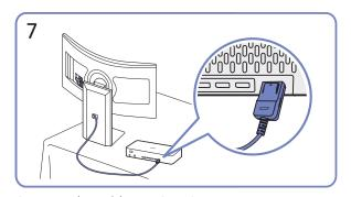
Connect the cables to One Connect.
