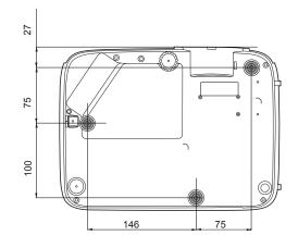
Ceilling/Wall Mount screw: M4 (Max. Length = 25 mm; Min. Length = 20 mm) Unit: mm
