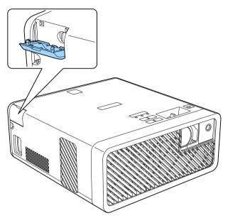
Connect the stereo headphone's mini-jack cable to the projector's Audio Out port.
