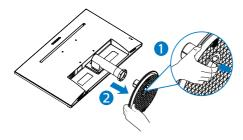
3. Press the release button to detach the base column.
